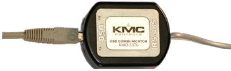
The USB (Universal Serial Bus) port is replacing the once common EIA-232 serial port that is now part of a legacy removal program in the computer industry. To replace the serial port as a network connection method, KMC Controls developed the KMD-5576 USB Communicator. The KMD-5576 is a USB to EIA-485 converter that directly connects a computer USB port to a KMC Tier 2 digital network by plugging into a controller or a NetSensor data port. Converter is shipped with cables and certified drivers.
