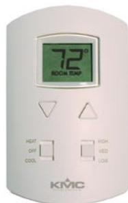
This is a temperature-sensing, wall-mounted, programmable operator interface for use in a KMC direct digital controls system. It includes intuitive-to-use setpoint buttons, and **two slide switches for heating/cooling change over and fan speed**. (Humidity is not sensed or displayed, and it does not have a hinged cover.) Four-pin EIA-485 data port on the underside allows temporary and easy direct communication with the connected controller via a local access port.
