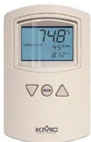
This is a temperature/humidity-sensing, wall-mounted, programmable operator interface for use in a KMC direct digital controls system. Three of its nine function keys can be reassigned by the user. Compared to the KMD-1161/1164/1181/1184, the KMD-1183/1185 has many similar features except that it has different button functions/labels:
