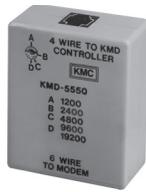
KMD-5550/5556 modem interfaces provide the communication link between **obsolete KMD-5501/5502/5504/5505** controllers or subnetworks with a modem to a compatible personal computer. They operate by converting EIA-485 signals from KMC equipment into the EIA-232 signals common to computer modem equipment and PC compatible computers. They operate with any Hayes™ compatible modem.
